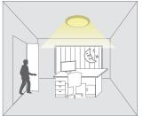
With movement and insufficient ambient lux level, the light is triggered on by the detector.
